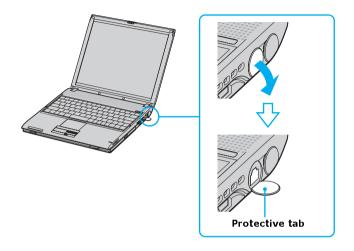
Gently pull the protective tabs away from the computer to find the Ethernet port and modem jack.
